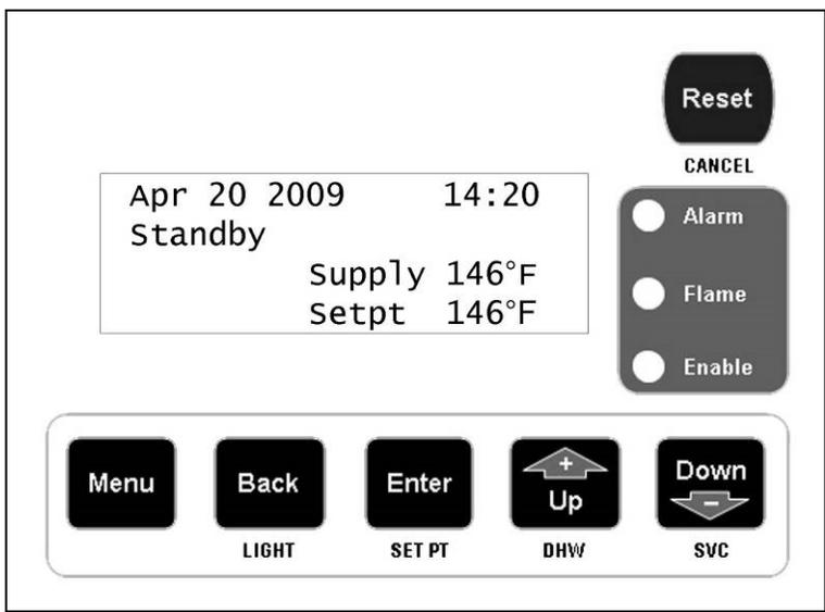
The display panel is used to setup and monitor boiler operation by means of six push buttons; MENU, BACK, ENTER, UP, DOWN, and RESET as shown.
