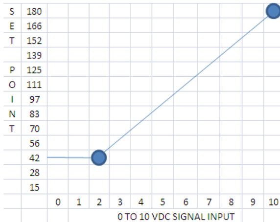
**NOTE:** When in analog control mode, enable/disable terminals are non-functional as the boiler is enabled/disabled by applying .5 to 1.5 VDC. Dropping below .5VDC will disable the boiler.
