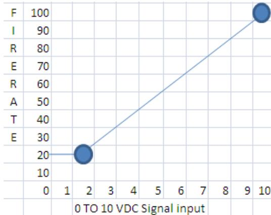
Boiler temperature limits and safety features are still active. Although the boiler may be receiving a 10 VDC signal, high fire will not be achieved if certain parameters, such as the boiler maximum temperature, are exceeded.
